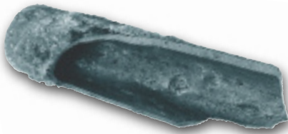
A fragment of corroded cast iron main
